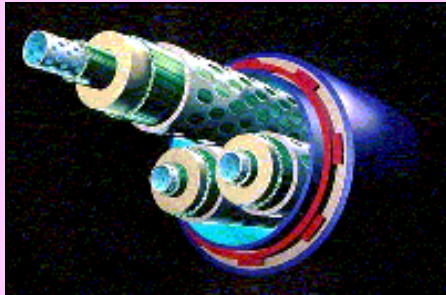
Concept and realization of a three-phase HTS power cable
