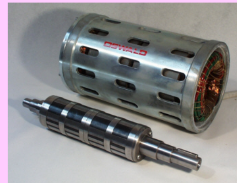
40kW 3000 rpm reluctance motor with YBCO bulk parts in the rotor
