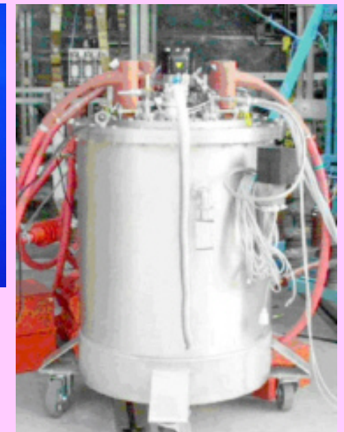
HTS fault current limiter based on melt-cast BSSCO
