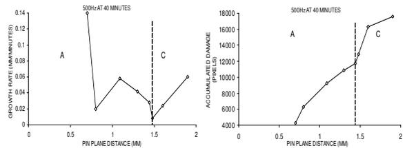
Figure 4 Accumulated damage and growth rate as a function of pin-plane distance showing the two regions A and C of tree growth.
