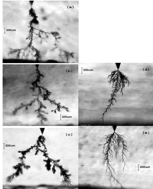
Figure 1 Captured photographs of tree growth for the XLPE cable samples prior to breakdown (a) 20Hz, (b) 50Hz, (c) 100Hz, (d) 300Hz and (e) 500Hz
