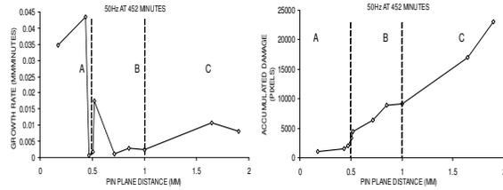
Figure 3 Accumulated damage and growth rate as a function of pin-plane distance showing the three regions A, B and C of tree growth.
