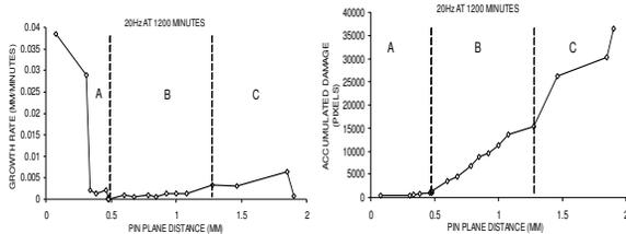
Figure 2 Accumulated damage and growth rate as a function of pin-plane distance showing the three regions A, B and C of tree growth.
