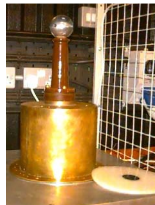
Fig. 1 Photograph of PEA electrodes system for thick plaque samples
