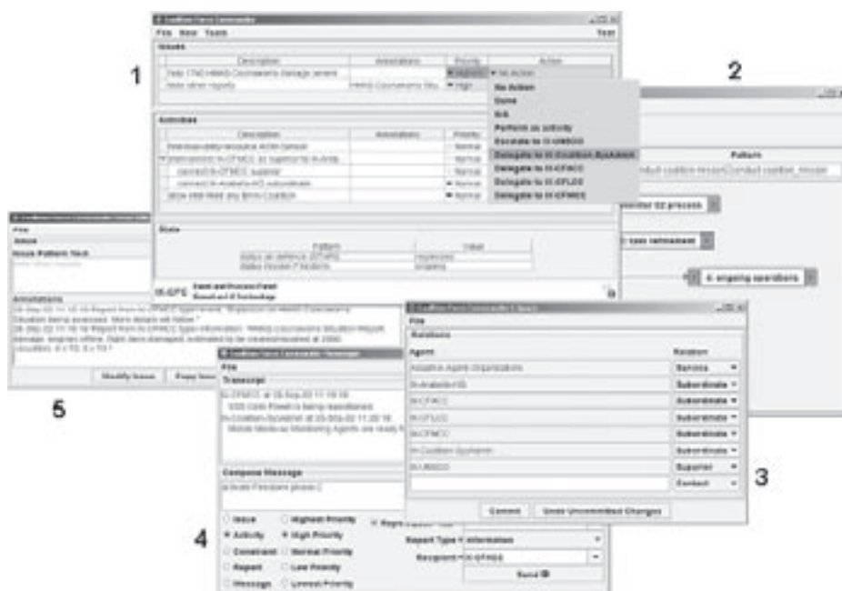
Figure 8: The I-X Tools include: 1. Process Panel (I-P2); 2. Domain Editor (I-DE): create and modify process models; 3 I-Space: maintain relationships with other agents; 4 Messenger: instant messaging tool, for both structured and less formal communications; 5 Issue Editor: create, modify, annotate issues.
