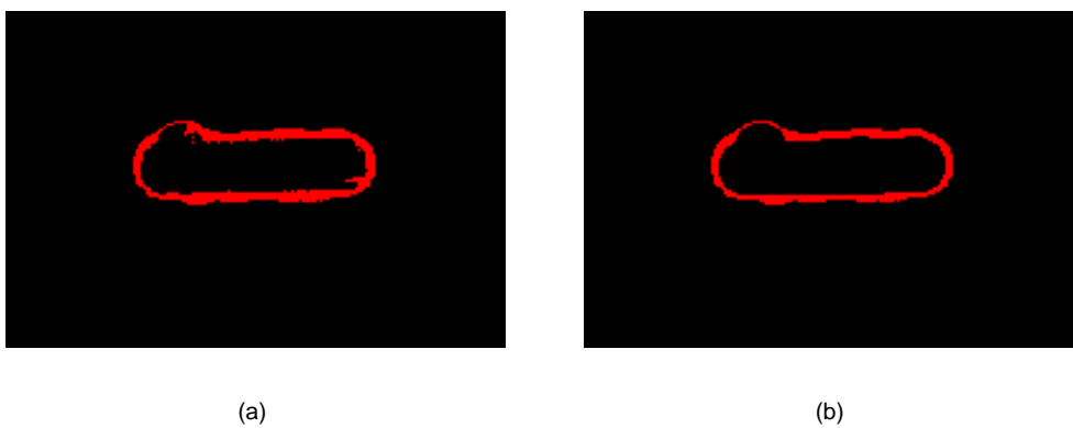
Figure 7.34: Misclassified pixels in the composite image of 100 frames using (a) image subtraction, (b) Hough transform.
