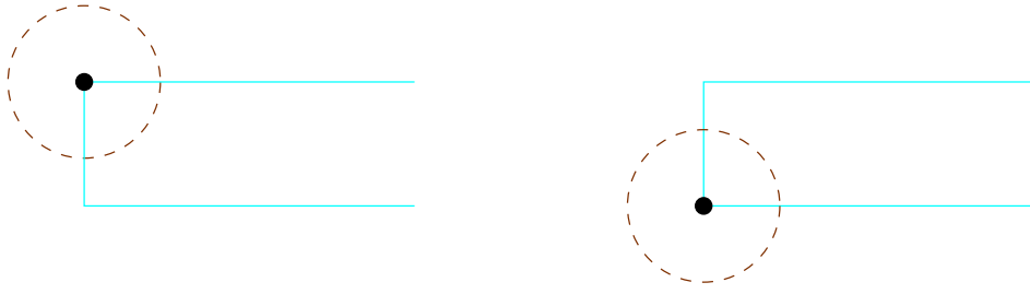
Figure 7.36: The distance between consecutive strips can be found using a pair of images from the captured video sequence. The Hough accumulator returns the centre and radius of the robot extracted from the image. Since the real world radius of the robot is also known, the real world distance between the two centres can be calculated.
