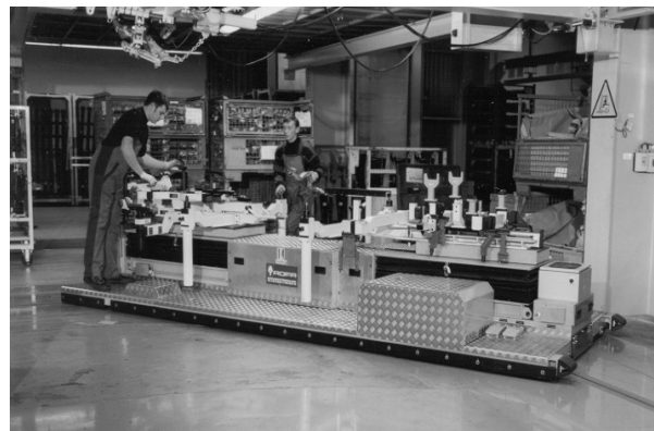
Fig. 1. A photograph of an ICPT moving platform applied in a vehicle fabrication line.
