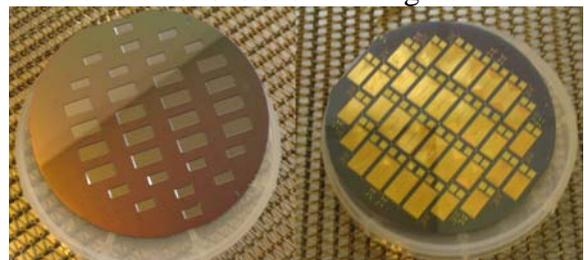
Figure 2. Diaphragms with Integrated Coils
