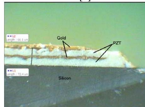
Figure 1. Cross-Section of 2 Layer PZT Actuator
