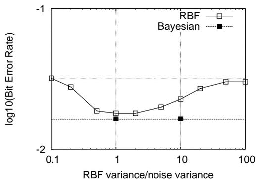
Figure 4: Influence of the RBF variance on the BER performance for transmission over the two-tap channel in conjunction with  $n_e = 2$  and  $\tau = 1$ , given SNR= 10 dB. The OFS aided FRCSM algorithm was used.
