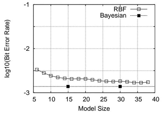
Figure 8: Influence of the model size to the BER performance for the three-tap channel with  $n_e = 4$  and  $\tau = 2$ , given SNR = 13 dB. The NLBER algorithm was used.
