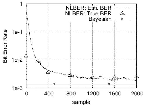
Figure 7: Learning curve of the NLBER algorithm averaged over 10 runs for the three-tap channel with  $n_e = 4$  and  $\tau = 2$ , given SNR = 13 dB.
