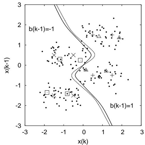
Figure 5: Comparison of the decision boundaries (solid: Bayesian and dashed: RBF) for the two-tap channel in conjunction with  $n_e = 2$  and  $\tau = 1$ , given SNR= 10 dB, where pairs of cross and plus symbols indicate the positions of symmetric state pairs, and the pairs of square and triangular symbols indicate the positions of RBF centre pairs. The OFS aided FRCSM algorithm was used.
