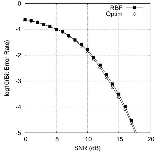
Figure 9: Comparison of BER performance for the three-tap channel with equaliser order  $n_e = 4$  and decision delay  $\tau = 2$ . The OFS with FRCSM algorithm was used.
