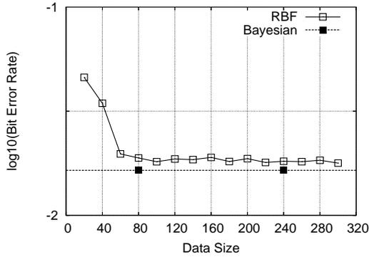
Figure 3: Influence of the data length on the BER performance for transmission over the two-tap channel in conjunction with  $n_e = 2$  and  $\tau = 1$ , given SNR= 10 dB. The OFS aided FRCSM algorithm was used.
