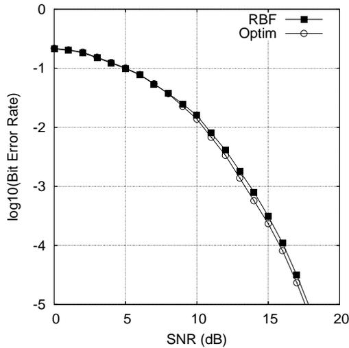
Figure 6: Comparison of BER performance for the three-tap channel with equaliser order  $n_e = 4$  and decision delay  $\tau = 2$ . The NLBER algorithm was used.
