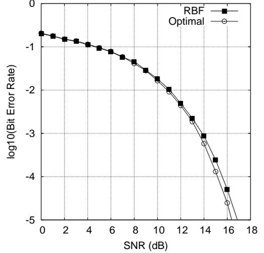
Figure 1: BER performance of the symmetric RBF and the Bayesian equaliser for transmission over a two-tap channel using an equaliser order  $n_e = 2$  and a decision delay  $\tau = 1$ . The OFS aided FRCSM algorithm was used.
