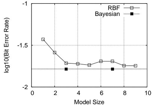
Figure 2: Influence of the model size on the BER performance for transmission over a two-tap channel in conjunction with  $n_e = 2$  and  $\tau = 1$ , given SNR = 10 dB. The OFS aided FRCSM algorithm was used.
