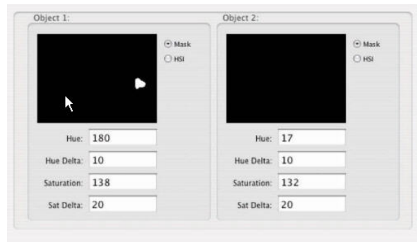
FIGURE 6.8: iGesture Reflexive Feedback Window. The white blob in the left window represents the purple object being tracked by the iGesture system.
