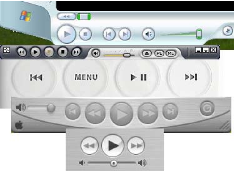
FIGURE 3.6: The picture shows many music player controls and their use of arrows to indicate the different controllers.
