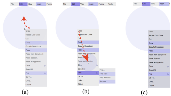
Figure 12. The extended design of bubbling menus. (a) When the user drags the right mouse button, a bubble appears that selects highlighted menu categories. A preview of the corresponding menu follows the cursor as the cursor’s center moves towards the menu bar. (b) The user moves the mouse downwards while dragging. The position of the menu freezes and a second bubble allows for the selection of highlighted items within the menu. (c) Alternatively, the user can release the button to activate the default view of a menu.
