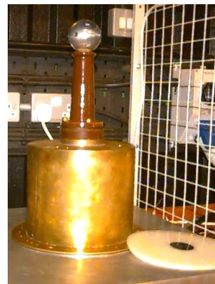
Figure 1. Photograph of the PEA electrodes system for thick plaque samples.
