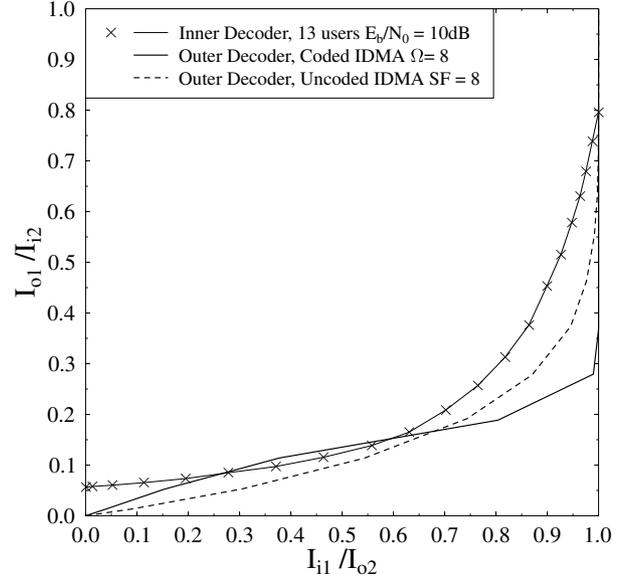
Fig. 3. EXIT chart analysis of coded IDMA over AWGN channels for a bandwidth expansion of  $\Omega = 8$ , 13 users and  $E_b/N_0 = 10\text{dB}$ .
