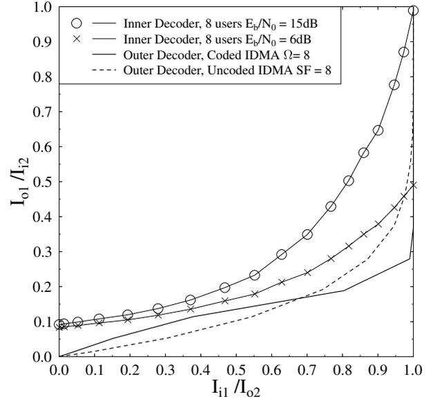
Fig. 2. EXIT chart analysis of coded IDMA over AWGN channels for a bandwidth expansion of  $\Omega = 8$ ,  $K = 8$  users and various  $E_b/N_0$  values.
