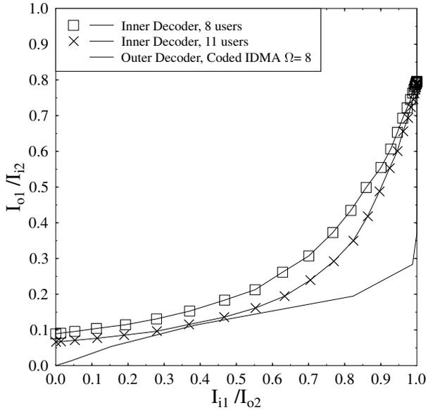
Fig. 4. EXIT charts for different number of users supported in coded IDMA over AWGN channels at a bandwidth expansion factor of  $\Omega = 8$  and  $E_b/N_0 = 10\text{dB}$ , using  $R = 1/2$  convolutional coding
