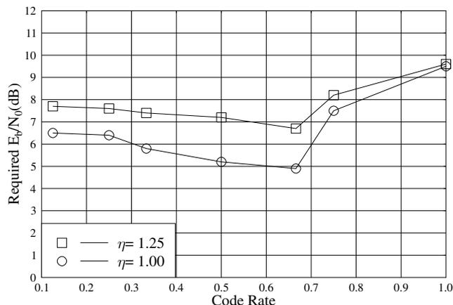
Fig. 6. The  $E_b/N_0$  values required for supporting a normalised user-load of  $\eta$  versus the code-rate at a fixed bandwidth expansion factor of  $\Omega = 8$  and for  $P_e = 10^{-5}$  using the convolutional codes of Table I
