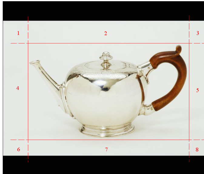
Figure 3.6: Showing bounding box in solid red and eight areas which a seed pixel of a new floodfill will be taken from
