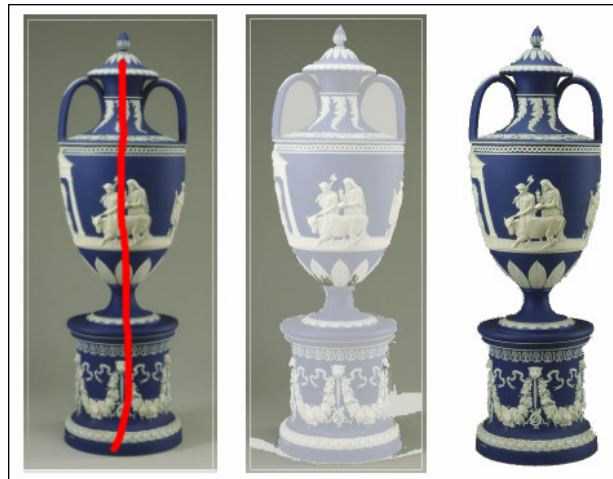
Figure 6.1: Showing the graduation from a bounding box and scribble, through the floodfill, and then with addition and subtraction of regions, and the final result.
