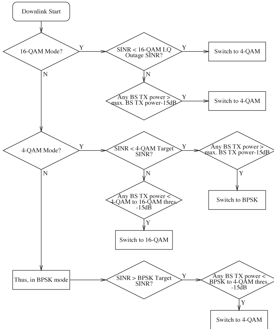
Fig. 5. AQAM mode switching algorithm used in the DL of the CDMA-based cellular network.
