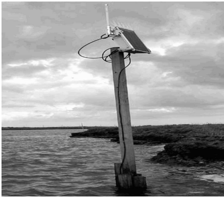
Figure 2: A FloodNET sensor node on site.
