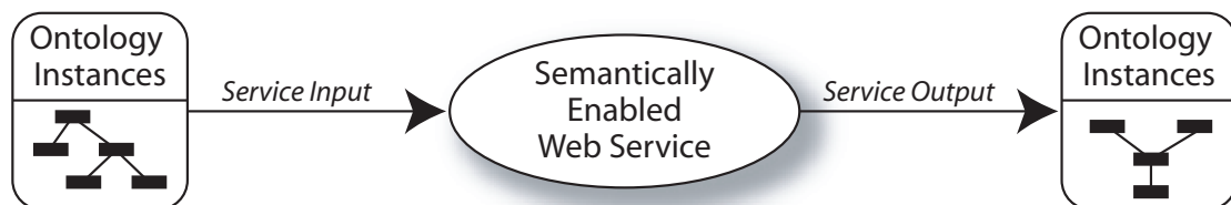
FIGURE 3.6: A Semantically enabled Web Service which consumes input and produces output in the form of ontology instances.
