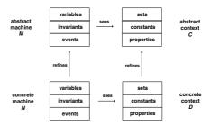
Fig. 2. Machine and context refinements
