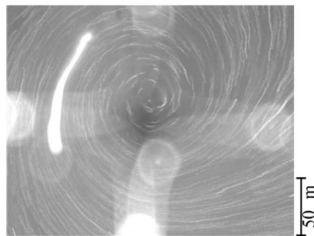
Figure 6. Top view of a rotating aqueous solution placed on top of four coplanar electrodes. Image of particle tracks obtained by superimposing successive video frames
