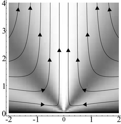
Figure 2. Streamlines and liquid speed for a vertically imposed temperature gradient. The gray levels indicate the magnitude of the liquid velocity, from zero (black) to maximum velocity (white)
