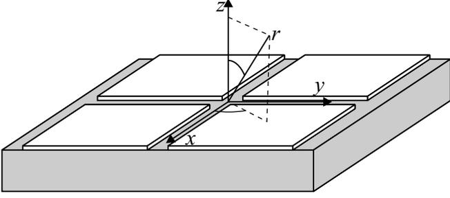
Figure 4. Schematic diagram of the four co-planar electrodes
