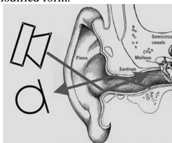
Figure 7 An ear signature is generated by probing the ear with a sound signal which is reflected and picked up by a small microphone [2]. The shape of the pinna and the ear canal determine the acoustic transfer function which forms the basis of the signature.
