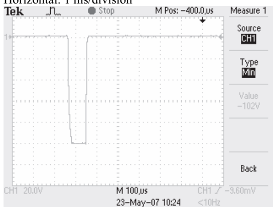
Fig 7 Output wave form of measured: Output voltage-102 Volts. Input voltage 100 V. Vertical scale: 20V/division Horizontal: 100μs/division
