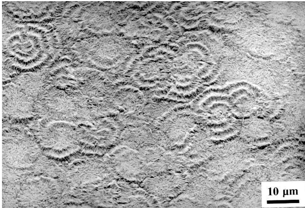
Figure 7.5(e): Banded spherulites with spacing \sim 2\text{ }\mu\text{m} form in BPA 118/20 M.
