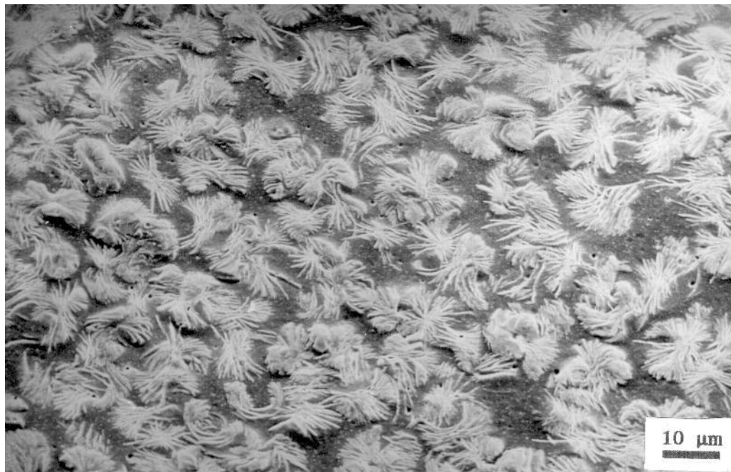
Figure 6.1(c): BPA 124/10 M showing compact lamellar aggregates.
