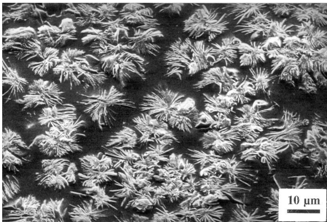
Figure 3.1(e): Small lamellar aggregates, 7% LPE blend crystallised at 124°C.
