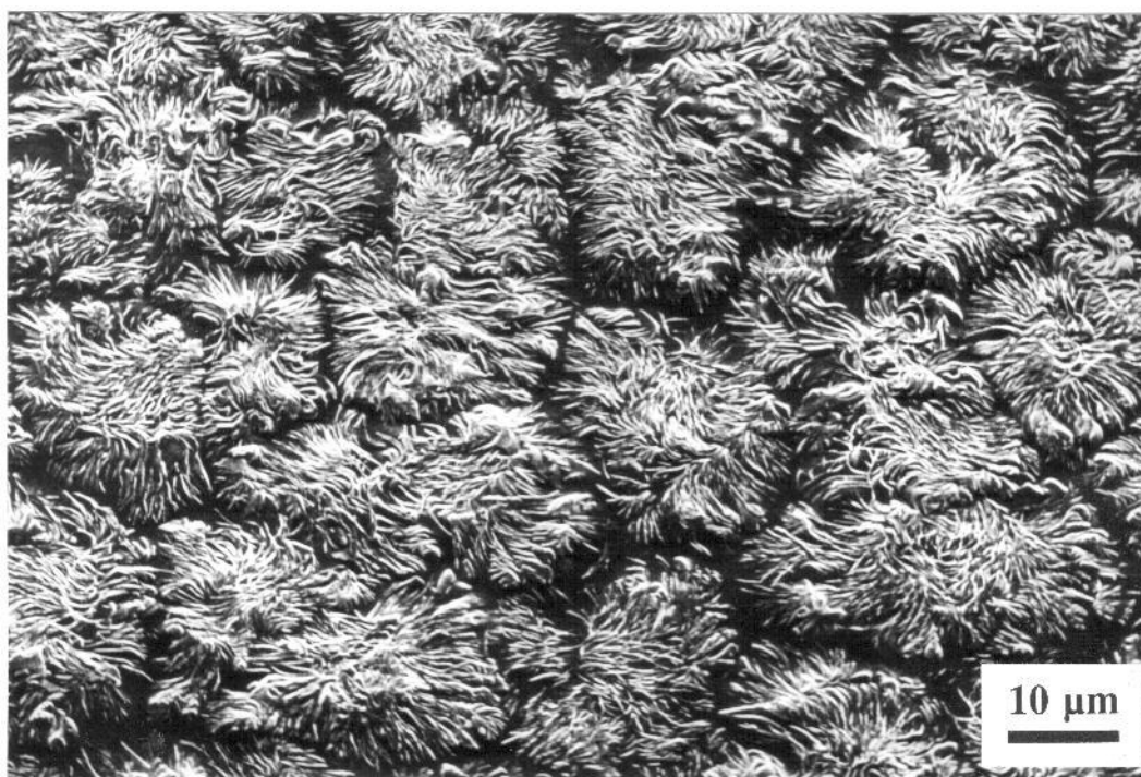
Figure 3.1(d): More compact lamellar aggregates, crystallisation 120°C.
