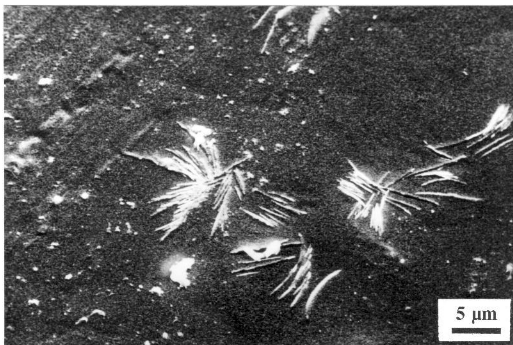
Figure 3.8(a): In BPA 124/1 isolated lamellar aggregates are formed.
