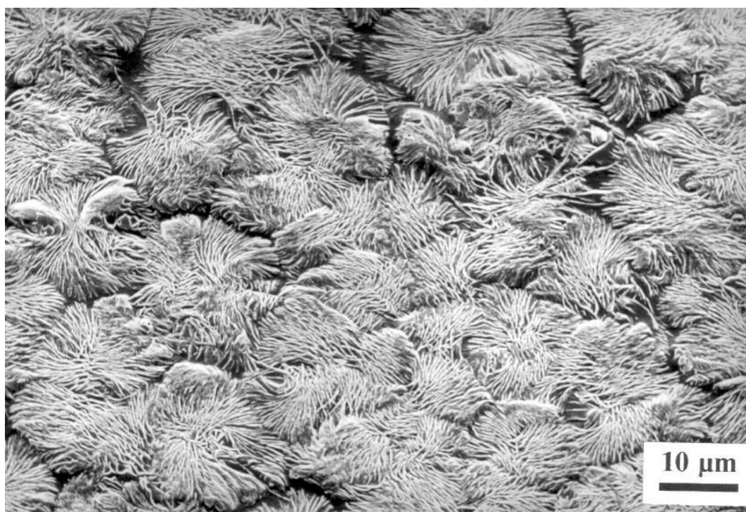
Figure 7.5(h): Compact lamellar aggregates in BPA 124/20 M.
