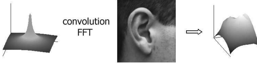
Fig. 8. Generating an ear energy surface by convolution. The energy field for an ear (right) is obtained by locating a unit value potential function (left) at each pixel location and scaling it by the value of the pixel and then finding the sum of all the resulting functions. For efficiency this is actually calculated in the frequency domain.
