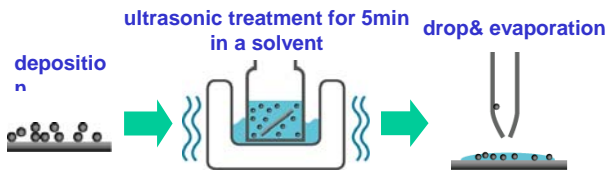
Fig. 2. A schematic flow-chart of the drop & evaporation process.
