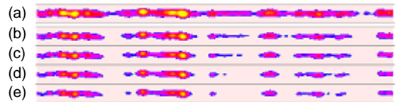
Fig. 6. Electron density distributions simulated for various Fermi energies. A mean donor concentration is 10^{20} \text{ cm}^{-3} .
