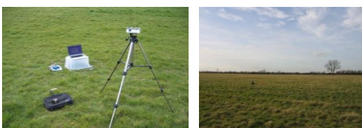
Prototype test apparatus. Ranging data recorded using a laptop computer, measurement referenced to measured distance in metres.
