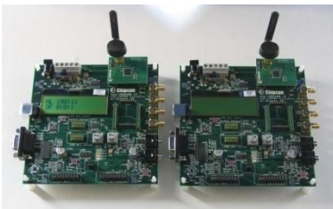
Chipcon CC2430 Development used to prototype RF-based TOF ranging algorithm.
