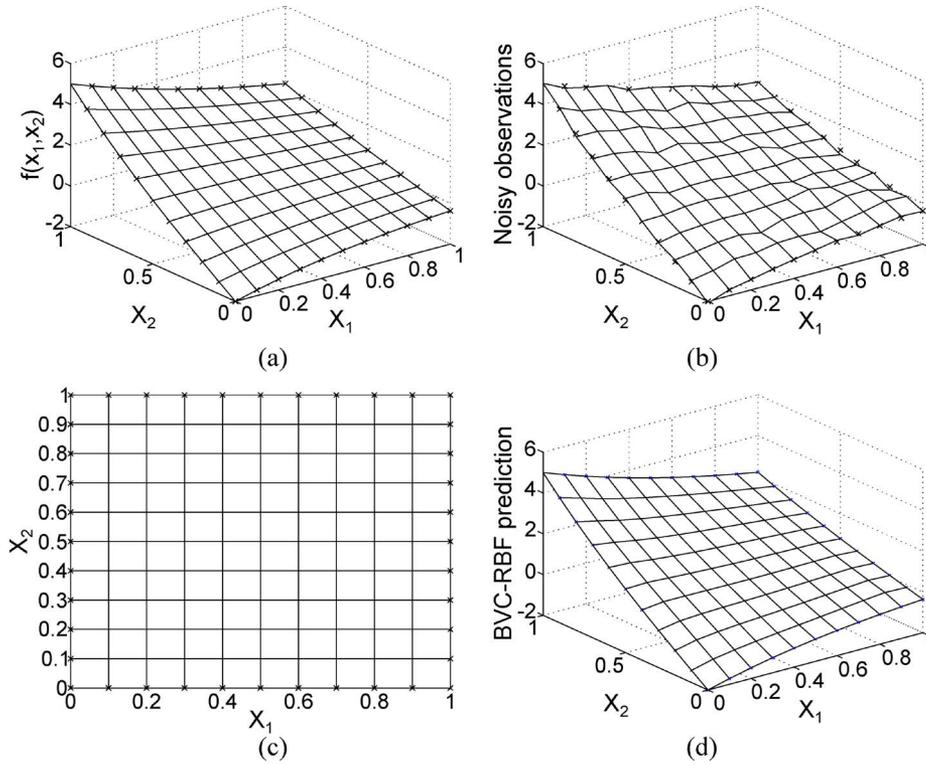
Fig. 3. Example 1. (a) True function  $f(x_1, x_2)$ . (b) Noisy data  $y(x_1, x_2)$ . (c) Boundary points. (d) Prediction of the resultant BVC-RBF model.
