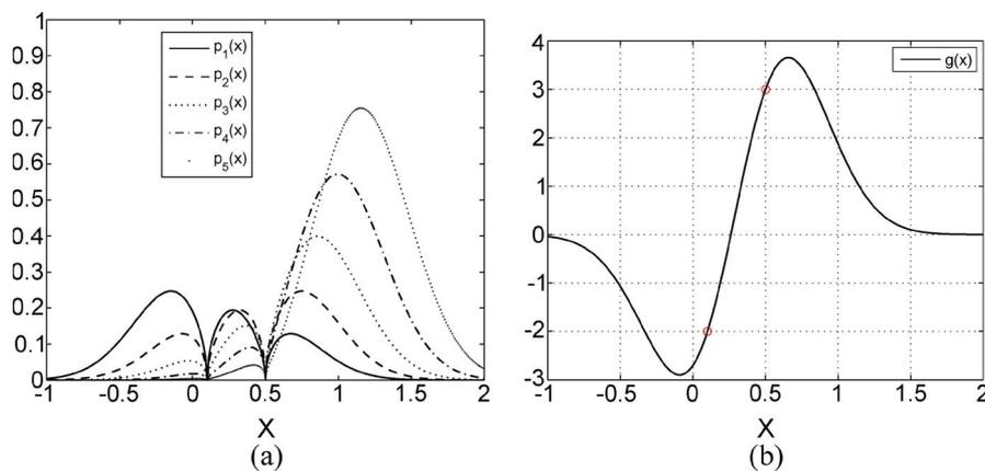
Fig. 2. Illustration of basis functions (a) zero forcing RBFs and (b) offset passing function  $g(x)$ .
