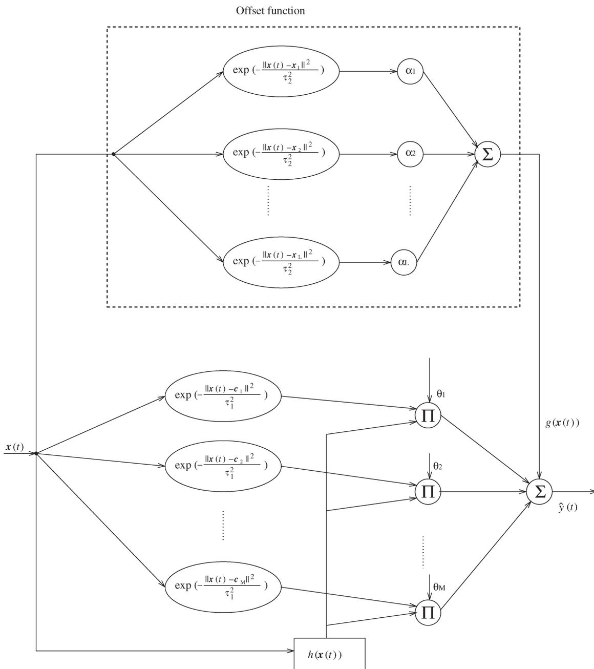
Fig. 1. Graphical illustration of the proposed BVC-RBF neural network.
