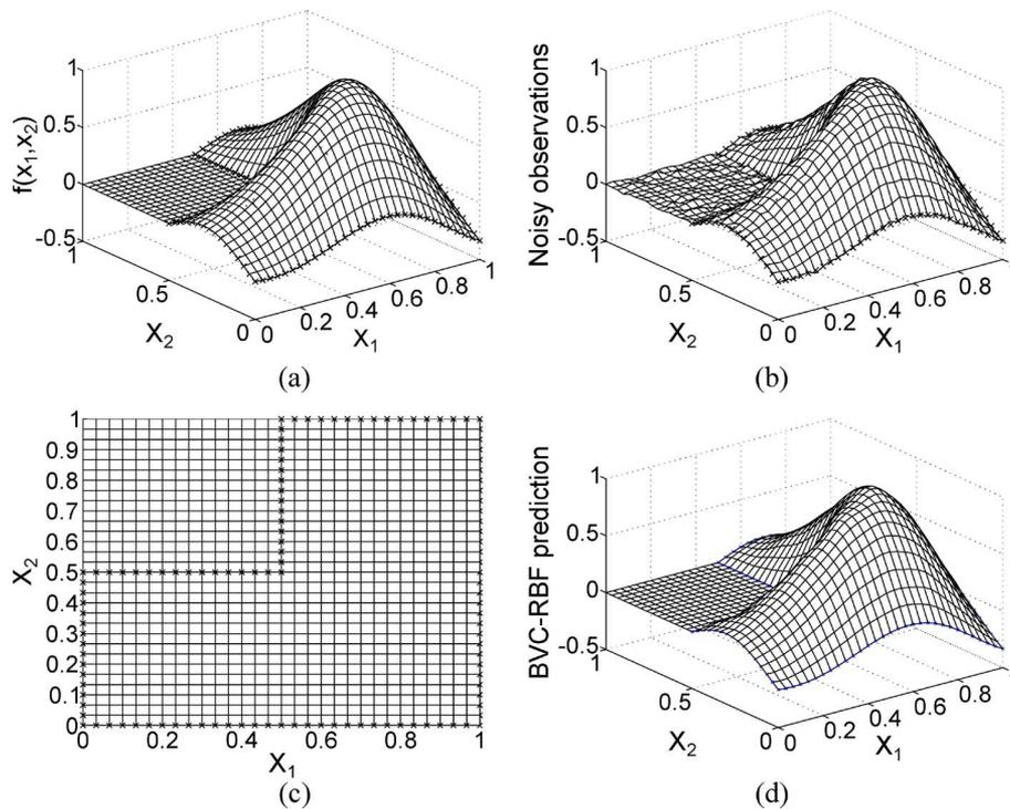
Fig. 5. Example 2. (a) True function  $f(x_1, x_2)$ . (b) Noisy data  $y(x_1, x_2)$ . (c) Boundary points. (d) Prediction of the resultant BVC-RBF model.
