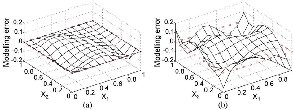
Fig. 4. Modeling error between the true function and the model prediction  $(\hat{y}(x_1, x_2) - f(x_1, x_2))$  for Example 1. (a) BVC-RBF model. (b) RBF model.
