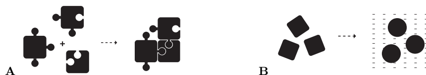
Fig. 1. Cartoon of the two basic biomolecular computing paradigms. In self-assembly computing (A) information is encoded by molecular shapes. Molecules with complementary shape form supra-molecular clusters through non-covalent binding. Thus shape-encoded input is mapped into features of the cluster as output. In conformational computing (B) the physicochemical environment of a macromolecule serves as input signal. Intramolecular dynamics maps this milieu information into a change in conformational state.
