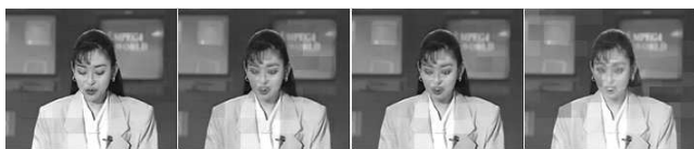
Fig. 7. Subjective video quality of the 45 th "Akiyo" video sequence frame using (from left) Rate- \frac{2}{3} , \frac{3}{4} , \frac{4}{5} and \frac{5}{6} SBCs of Algorithm-I summarised in Table I at E_b/N_0=0.5 dB.
