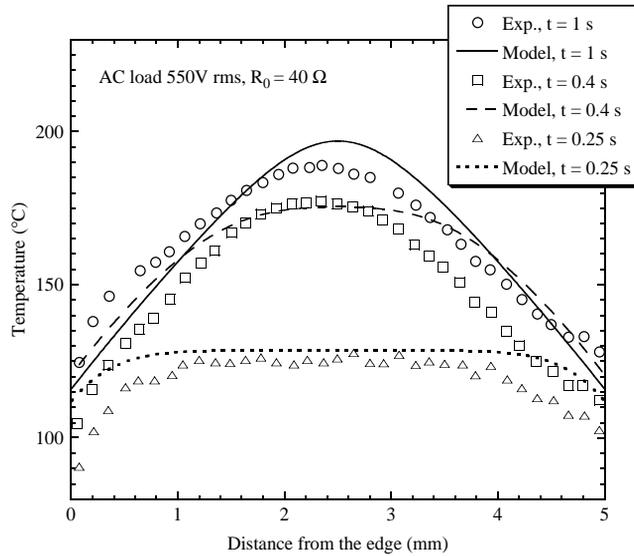
**Figure 4.** Comparison of numerical predictions of temperature field in a thermistor at different time instants with surface thermography
