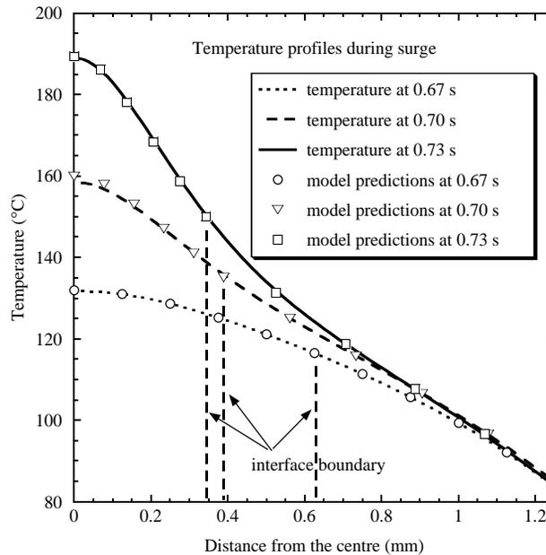
**Figure 5.** Numerical predictions for temperature distribution in a thermistor at different time instants of the surge stage using the front-fixing technique
