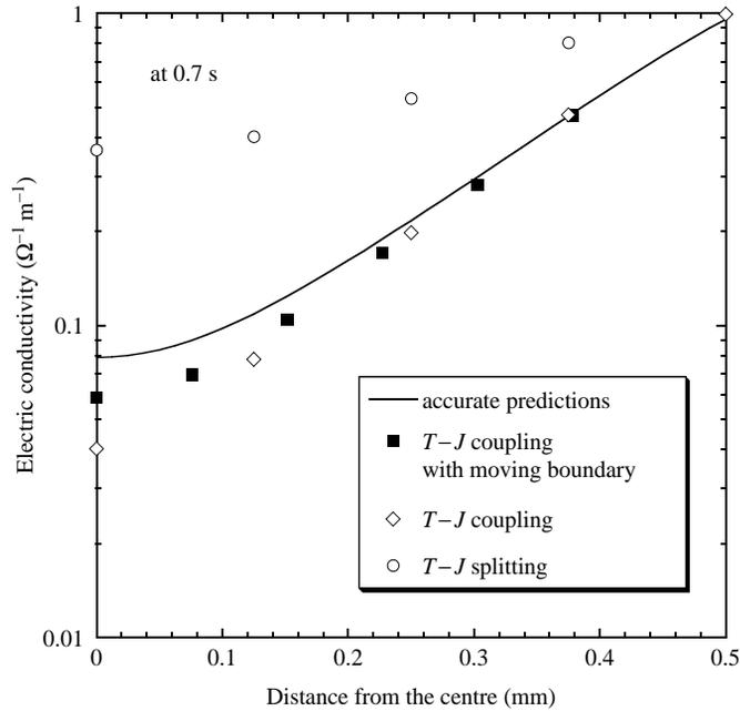
**Notes:** A mesh with 10 space intervals was used and the time step of 20ms was taken. Coupled treatment provides high accuracy
