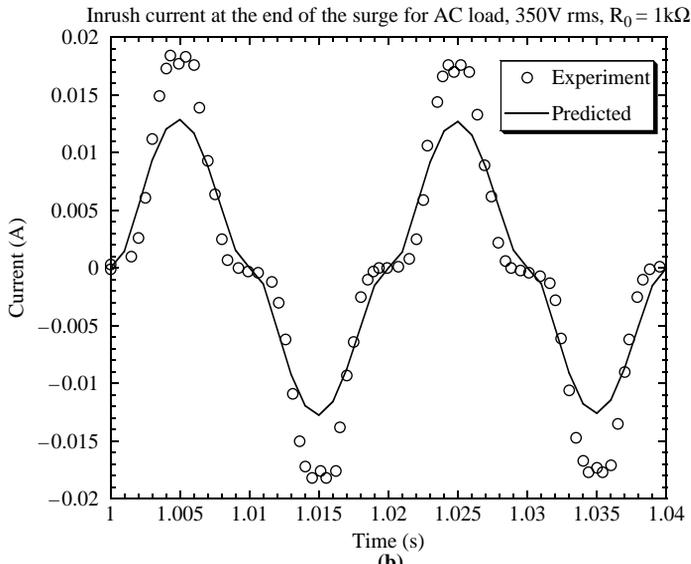
**Notes:** Test calculations were done on a fine uniform grid (100 intervals) with a small time step 0.1 ms
