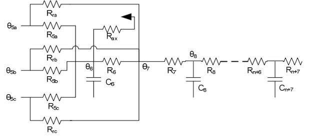
**Figure 2 – Equivalent thermal network of tunnel** and radiation heat transfer must be considered at nodes 6 (representing the tunnel air) and 7 (representing the tunnel wall) respectively. The equivalent thermal network for the case of one circuit is shown in Fig 2. The left hand side of Fig. 2 shows the connection to node 5 at the outer edge of the cable. The method does not pose a limit on the number of independent cables for which a temperature distribution can be obtained.
