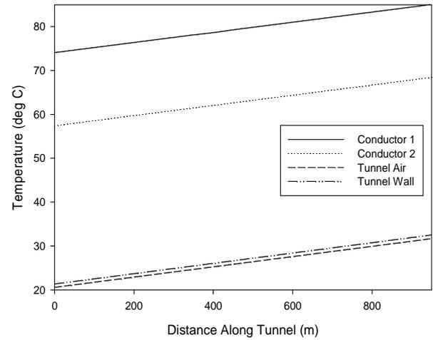
**Figure 3 – Temperature profile for steady state rating calculation**
