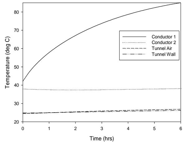
**Figure 4 – Temperature Profile for 6hr emergency rating calculation**
