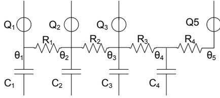
**Figure 1 – Equivalent thermal network of cable**
