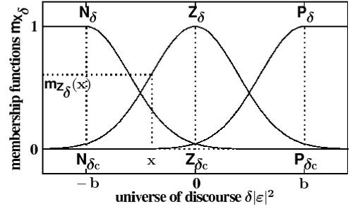
Fig. 3. Membership functions over the universe of discourse for  $\delta|\varepsilon_n|^2$ , where the fuzzy variable  $X = N, Z$  or  $P$ .
