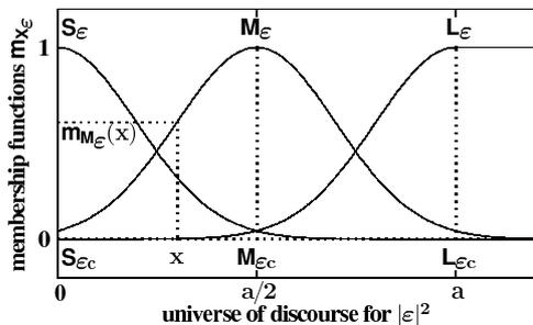
Fig. 2. Membership functions over the universe of discourse for  $|\varepsilon_n|^2$ , where the fuzzy variable  $X = S, M$  or  $L$ .
