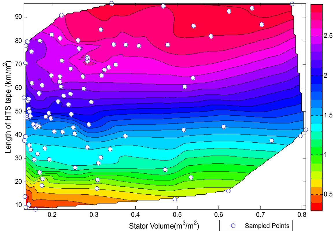
Fig. 2 Achievable air-gap flux density in a full size machine as a function of the quantities of stator iron and HTS tape used. These quantities are expressed per unit air-gap surface area.
