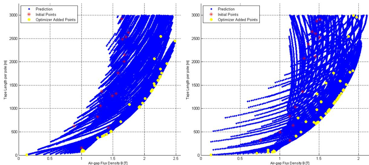
Fig. 5. Achievable air-gap flux density with iron poles on the rotor core and HTS winding at 40 K, as a function of the quantity of HTS tape used. The results on the right were obtained with larger allowances around the coils.
