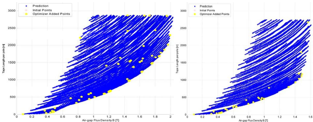
Fig. 4. Achievable air-gap flux density with an inner rotor core and HTS winding at 40 K, as a function of the quantity of HTS tape used. The results on the right are for the smaller rotor radius.
