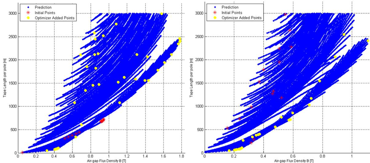
Fig. 3. HTS tape requirements and achievable air-gap flux densities for various coreless rotor designs with a slotless stator, with the winding at 40K (left) and at 60K (right).
