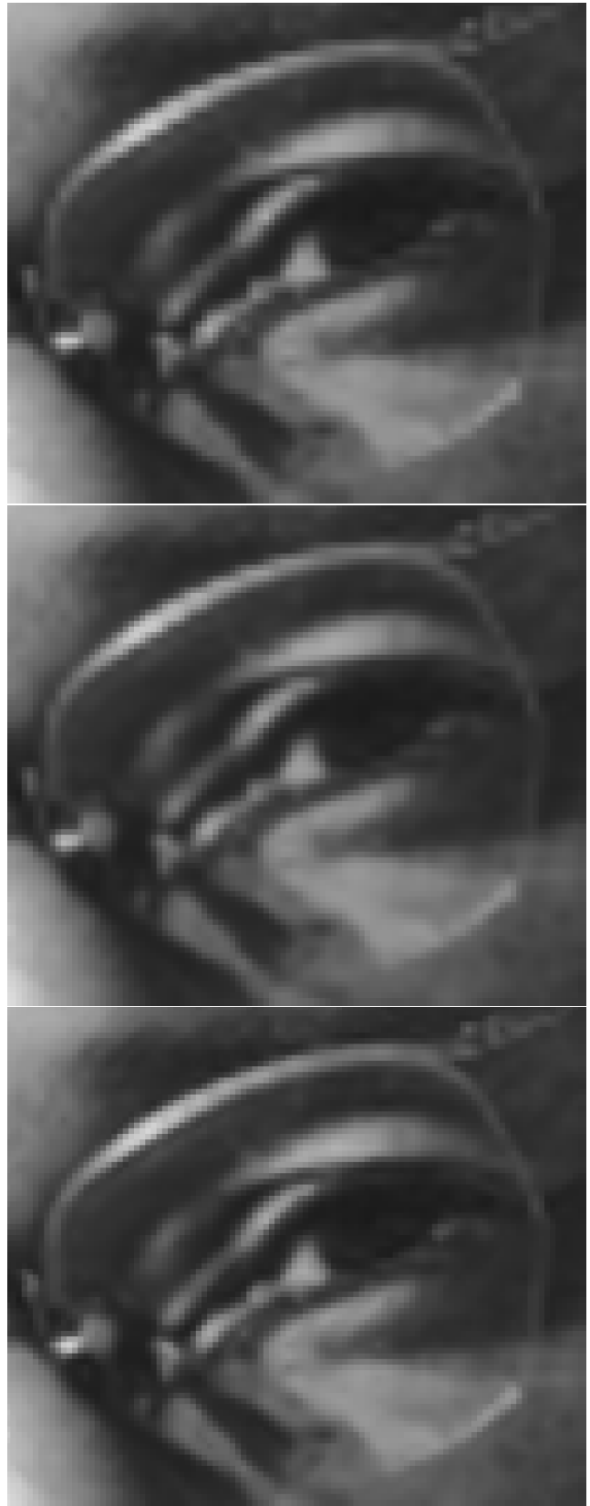
Figure 1: 103x89 crops of enlargements of a low-noise 64x64 pixel image to 127x127: monotone bicubic splines (top), Nohalo (middle) and ICBI.
