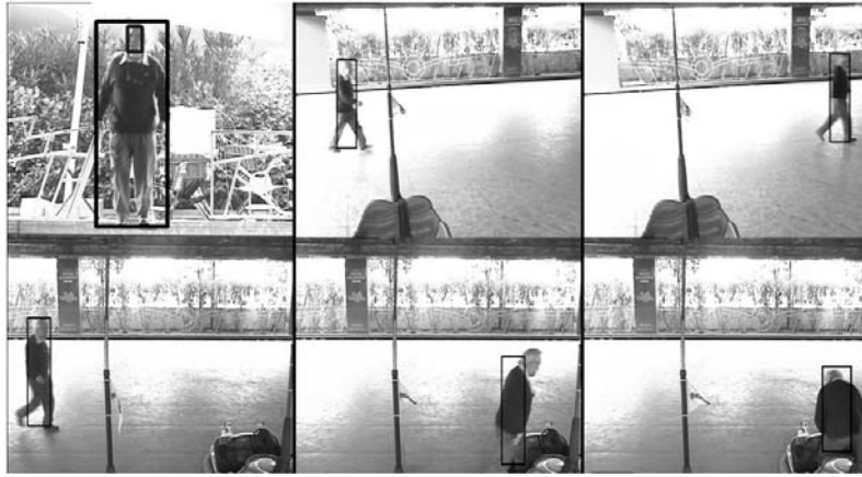
Fig. 10. Recognition and multicamera tracking. Initially the face is detected and the visitor recognised (i-cam). A hand-off between the i-cam and the t-cam1 camera takes place. The handoff between the t-cam1 and the t-cam2 follows. The visitor is associated to the bumper car in which he enters.
