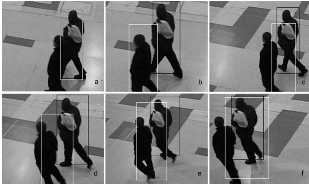
Fig. 5. Tracking Results - PETS Sequence: White PF, Black PM, 100 particles, frames 1,15,30,45,60,75.
