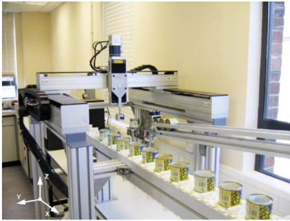
Fig. 1. Multiaxis gantry robot with the axes marked.
