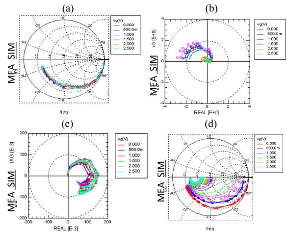
Fig. 3 Fitting of (a) S11, (b) S12, (c) S21, (d) S22 parameter curves of the short channel device with  $V_{GS}=0, 0.5\text{V}, 1.0\text{V}, 1.5\text{V}, 2.0\text{V}, 2.5\text{V}$  and  $V_{DS}=50\text{mV}, 0.5\text{V}, 1.0\text{V}, 1.5\text{V}$  (orders not shown).
