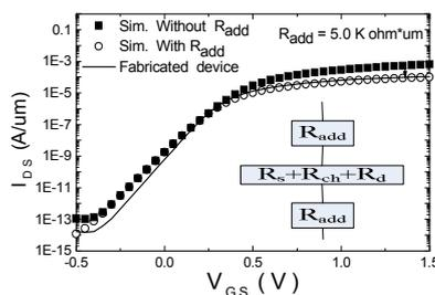
Fig. 5  $I_{DS}$  vs.  $V_{GS}$  with  $V_{DS}=1.5\text{V}$ .
