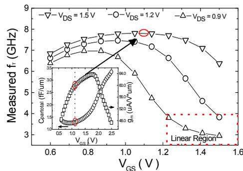
Fig. 7 Measured  $f_T$  vs.  $V_{GS}$  with  $V_{DS}=1.5, 1.2, 0.9\text{V}$ .
