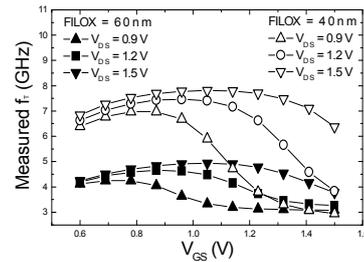
Fig. 6 Measured  $f_T$  vs.  $V_{GS}$  for 100nm DGC devices.
