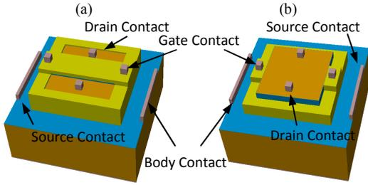
Fig. 8 3D structures of FGC and DGC devices.
