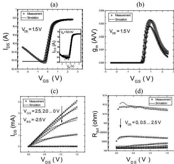
Fig. 1  $I_D$ - $V_G$  and  $g_m$ ,  $I_D$ - $V_D$ , output resistance curves of the short channel device with  $V_{DS}=0.5\text{V}$  and  $1.5\text{V}$  in (a) (b) and  $V_{BS}=-2.5\text{V}$  in (c) (d).
