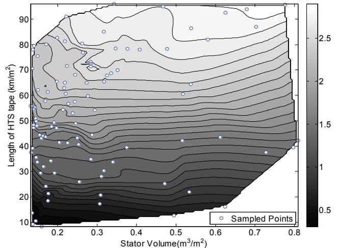
Fig. 2 Achievable air-gap flux density in a full size machine as a function of the quantities of stator iron and HTS tape used. These
