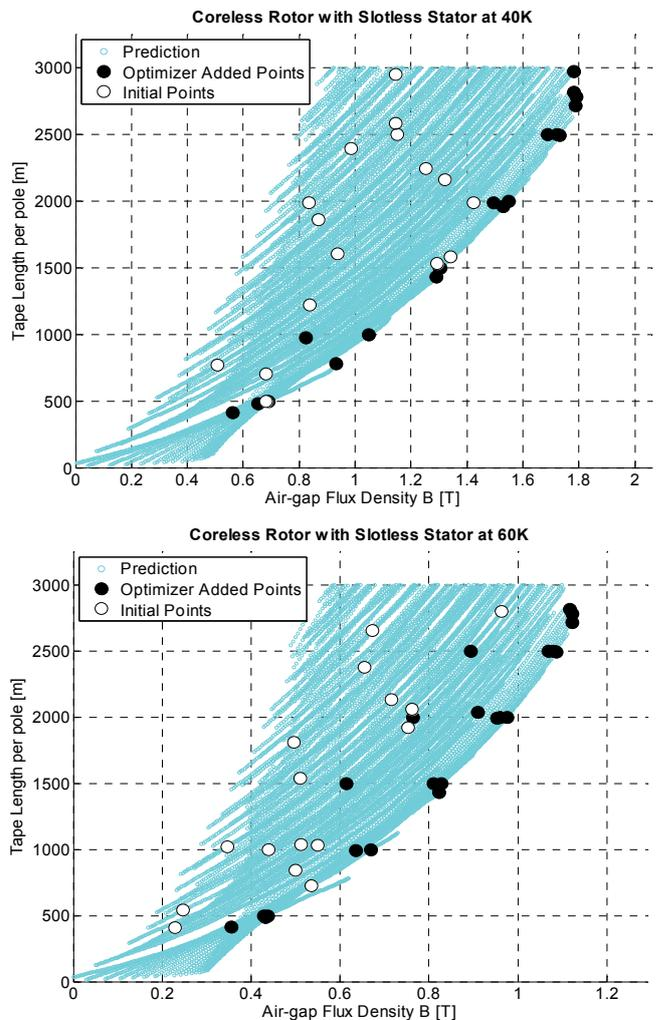
Fig. 3. HTS tape requirements and achievable air-gap flux densities for various coreless rotor designs with a slotless stator, with the winding at 40K (upper) and at 60K (lower).
