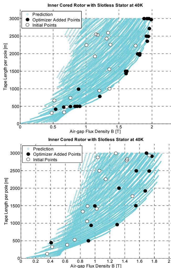
Fig. 4. Achievable air-gap flux density with an inner rotor core and HTS winding at 40 K, as a function of the quantity of HTS tape used. The results at the bottom are for the smaller rotor radius.
