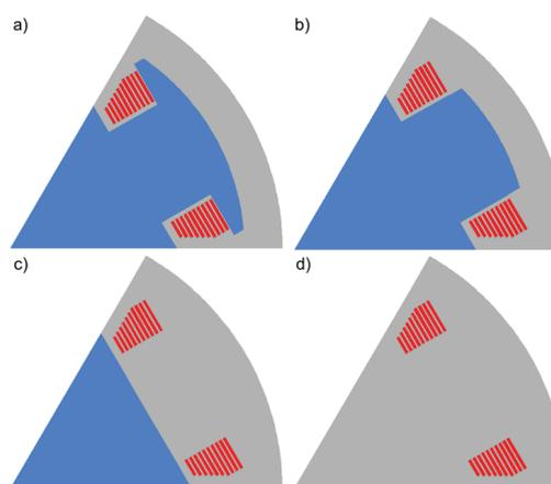
Fig.1. Rotor configurations chosen for the design study: a) fully cored, b) inner core and coil core, c) inner core, d) fully coreless
