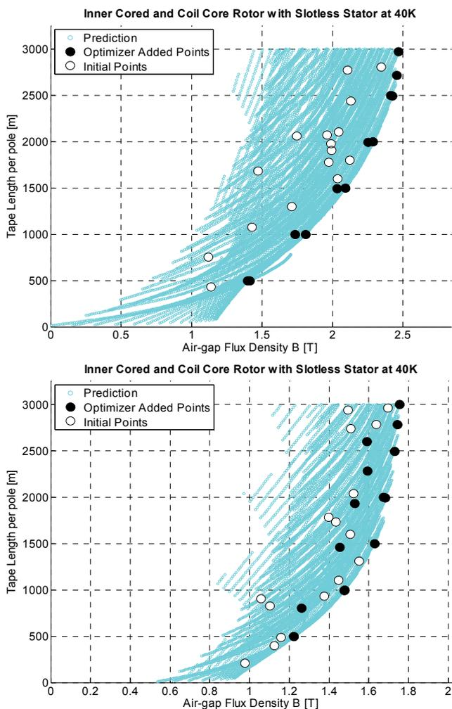
Fig. 5. Achievable air-gap flux density with iron poles on the rotor core and HTS winding at 40 K, as a function of the quantity of HTS tape used. The results at the bottom were obtained with larger allowances around the coils.
