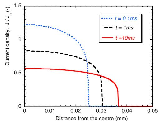
Fig. 2. Evolution of current density  $J_z(r, t)$  in a HTS circular wire. The analytical prediction of electric field and current density for a wire with  $I_0 = 2\text{A}$ ,  $R=0.5\text{mm}$  and  $\alpha=6$  is shown at different instances of time.
