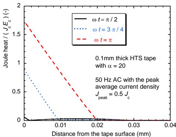
Fig. 1. Typical variation of Joule heat release in HTS tapes under AC load at different instants during the cycle.
