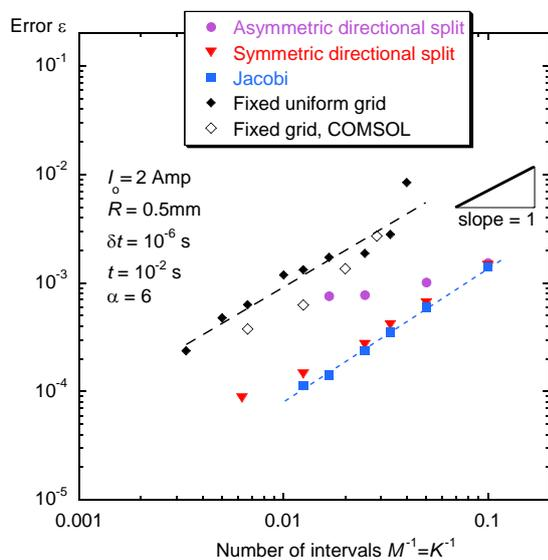
Fig. 3. Numerical prediction of an electric field  $E_z(x,y)$  for a wire with  $I_0 = 2$ A,  $R=0.5$ mm and  $\alpha=6$  after  $t = 10$  ms: the mesh size effects. Errors in predictions reveal an approximately first order of accuracy  $O(M^{-1})$ .
