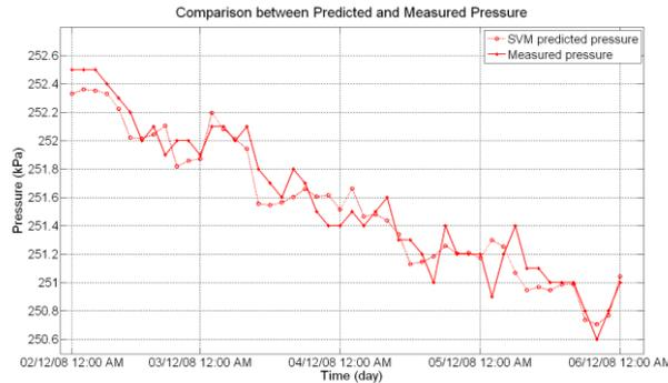
Figure 1: Predicted pressure on training data and measured pressure for cable 1\_1\_R\_A\_NC.
