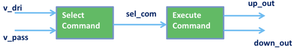
Fig. 1. RRM diagram showing initial abstract representation of power window model
