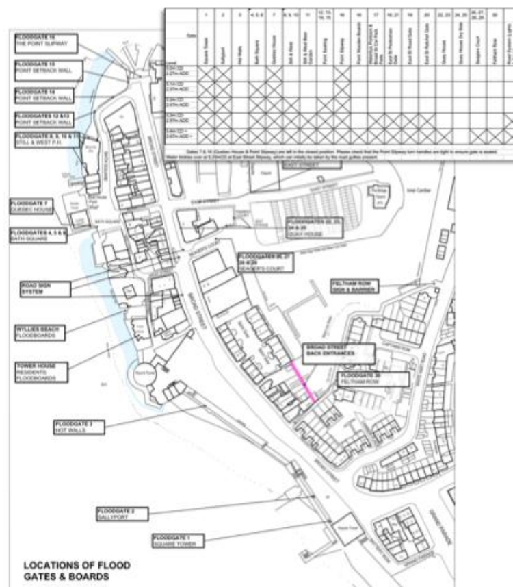
Figure 7-3 Locations of floodgates in Portsmouth, shown with the sequence in which they are closed during a flood (photograph courtesy CDP)
