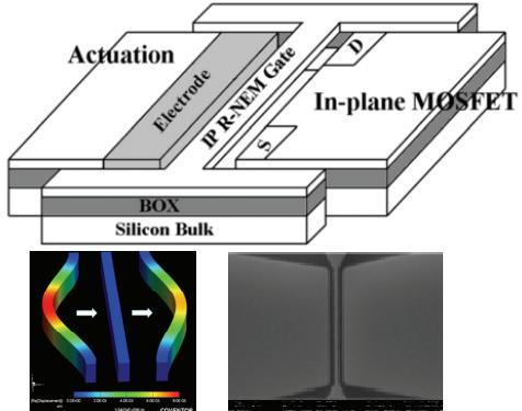
**Fig.7** A schematic diagram of IP-RSGFET.
