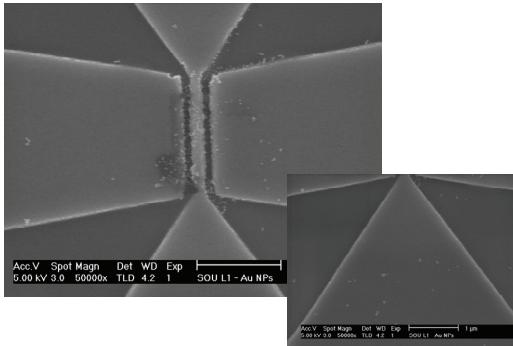
**Fig.2** A SEM image of a AuNP coated SiNW with selectively  $\text{NH}_2\text{SAM}$  functionalized surface.
