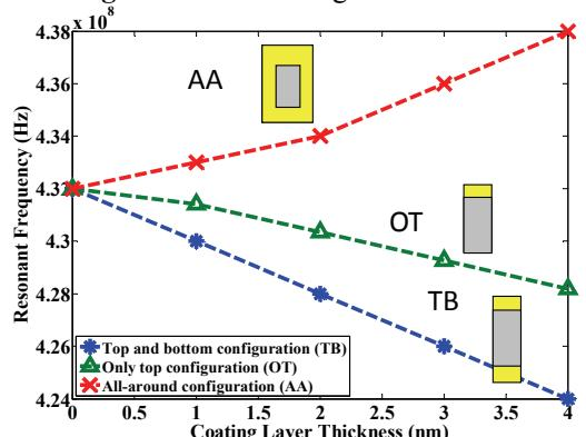
**Fig.8** Resonance frequency vs surface coating layer thickness calculated for three different coating configurations..
