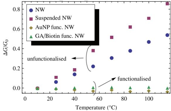
**Fig.5** Normalized temperature dependence of conductance variation for various SiNWs..
