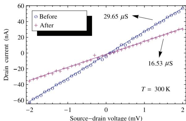
**Fig.4** I-V characteristics at 300K for SiNW before and after  $\text{NH}_2\text{SAM}/\text{GA}/\text{Biotin}$  functionalization..
