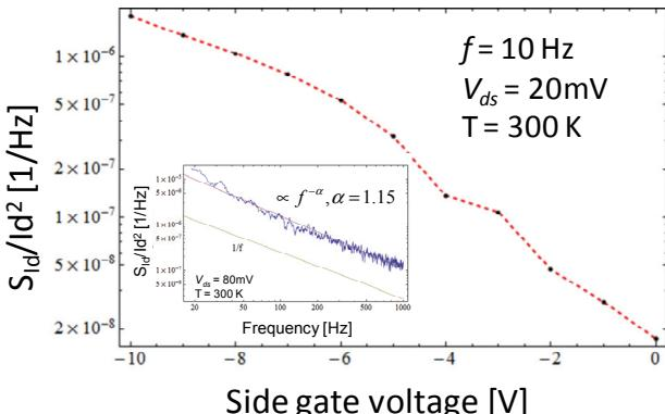
**Fig.6** LF noise intensity as a function of side gate voltage. The inset shows LF noise spectrum.
