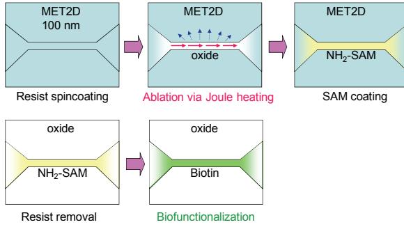
**Fig.1** Selective  $\text{NH}_2\text{-SAM}/\text{GA}/\text{Biotin}$  functionalisation procedure by Joule heating method.
