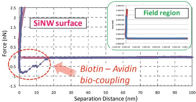
**Fig.3** Force-distance curve observed for avidin-functionalized AFM tip and biofunctionalized SiNW. The inset shows the curve for unfunctionalized field region.
