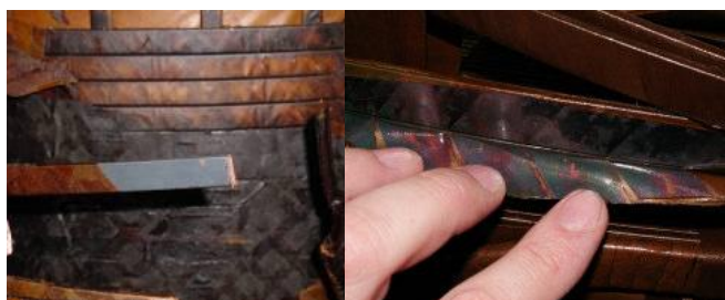
Figure 1: Conductor and papers from the inspection of a failed unit [1].
