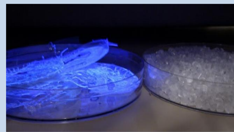
Fig. 1. Comparison between polystyrene doped with pyrene (5%wt.) and unmodified polystyrene.
