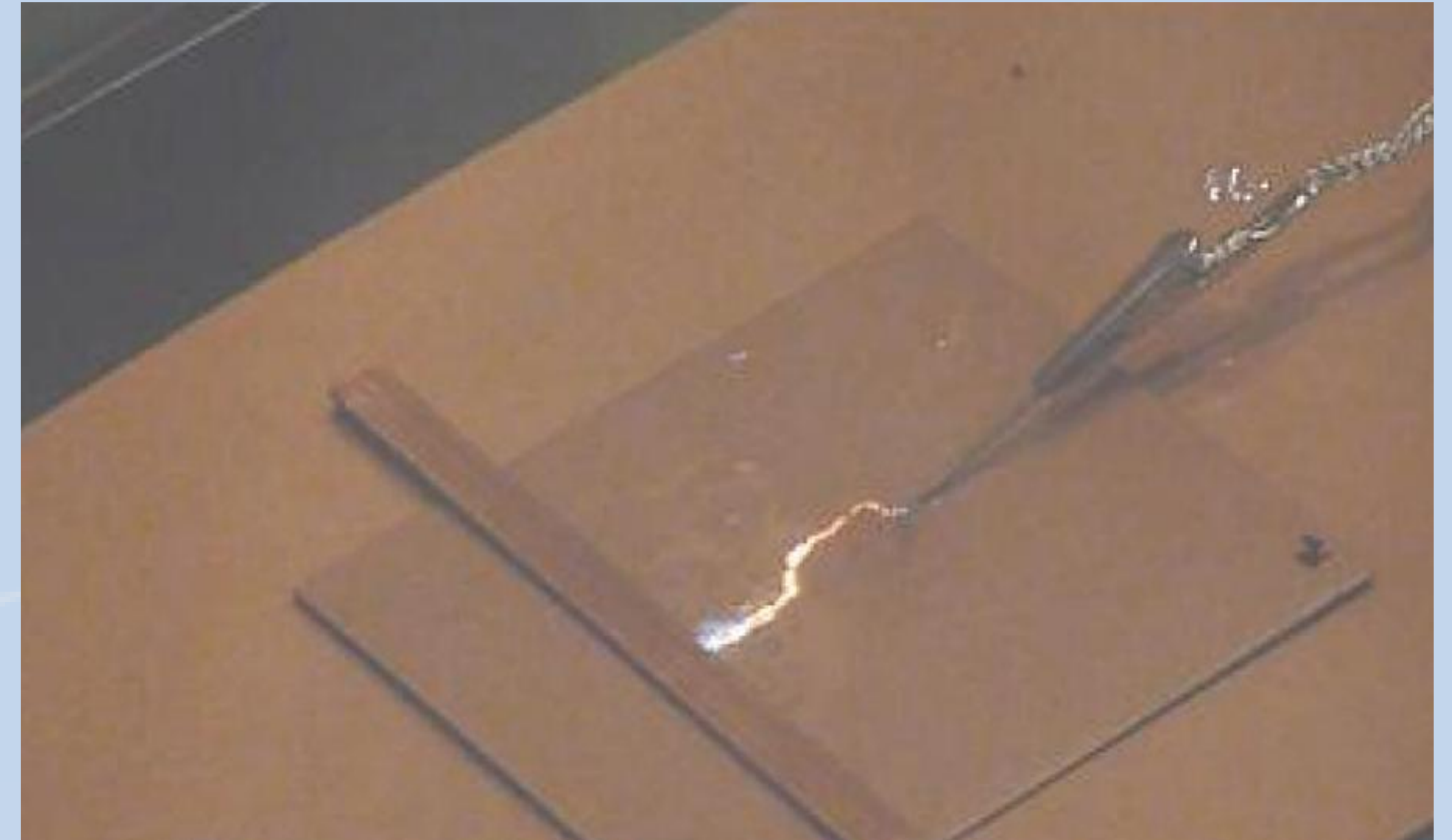
Figure 3: Example of a full-length discharge without tripping the protection system (overcurrent protection is set to 20mA – HV side current)
