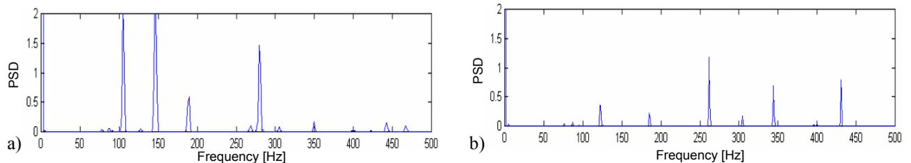
Figure 8 PSD of an impact test, grinding wheels pressing on blade (a) and off (b)
