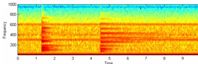
Figure 7 Impact test spectrogram, grinding wheels pressing on blade and off
