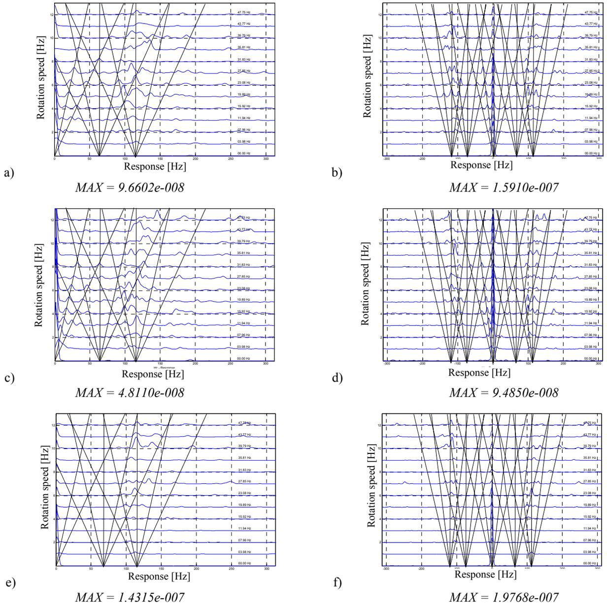
Figure 4 Single grinding wheel sharpening: one sided cascade plot for (a)  $DC=100$ , (c)  $DC=10$ , (e)  $DC=1$  and corresponding two sided plots (b-d-f)
