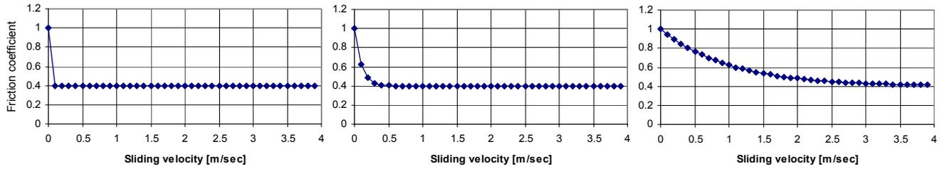
Figure 2 Friction coefficient curve:  $DC=100$ ,  $DC=10$  and  $DC=1$
