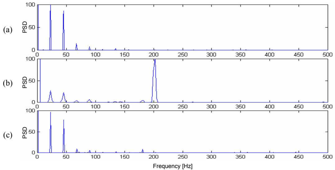
Figure 9 PSD of a short sharpening test: (a) before, (b) during and (c) after sharpening
