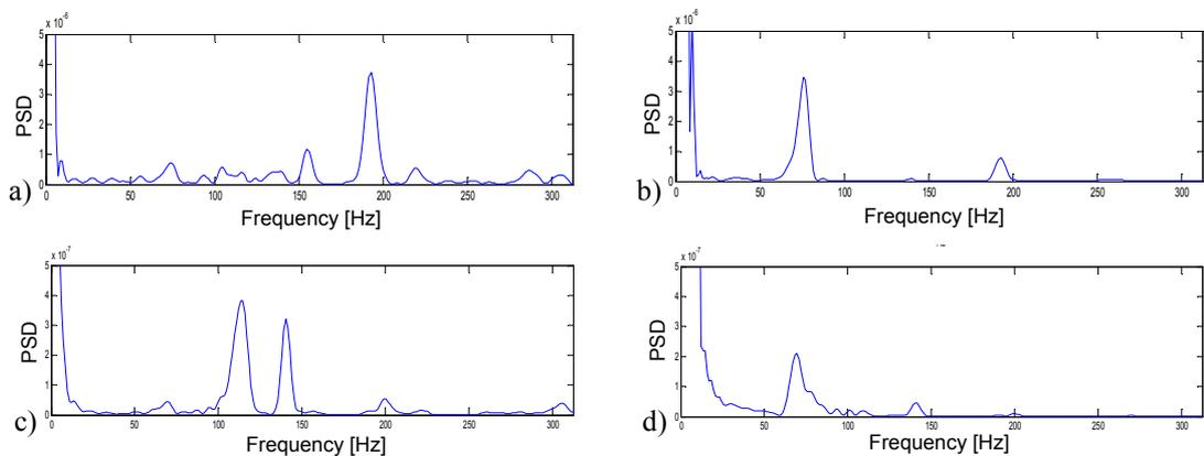
Figure 3 PSD of impact simulation for non-rotating disk blade for the systems with one (a, b) and two grinding wheels (c, d): corresponding to a peripheral node of the disc blade (a, c) and to a node of the grinding wheel (b, d)
