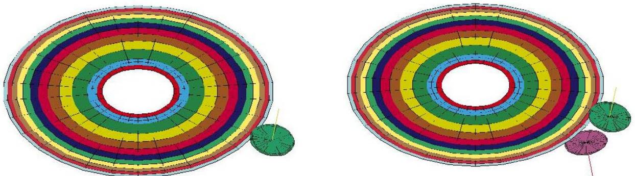
Figure 1 Disk blade model with one and two grinding wheels
