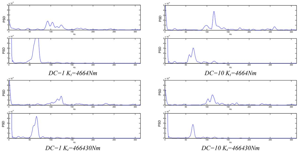
Figure 6 PSD of the disk edge (above) and of the grinding wheel (below) related to sharpening simulations with a torsional spring added to the axis of the disk model (145 rad/sec angular speed)
