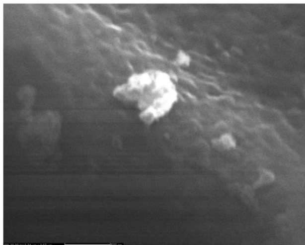
Figure 74. The surface of an SU-8 particle imaged by electron microscopy showing a pitted, porous surface. Scale bar represents 500 nm
