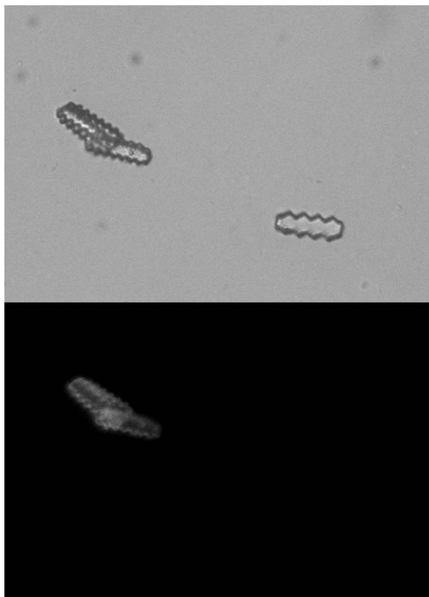
Figure 81. White light and fluorescence images of two encoded particle types (with all four types present in the assay). Three type 3 encoded particles functionalised with probe (PL) are visible on the left of the images along with a single type 2 encoded particle with probe (PK). Particles had been exposed to 20 nM labelled target (TI) at 54°C, the image shows the discrimination between complementary sequences and those mismatching by a single base-pair
