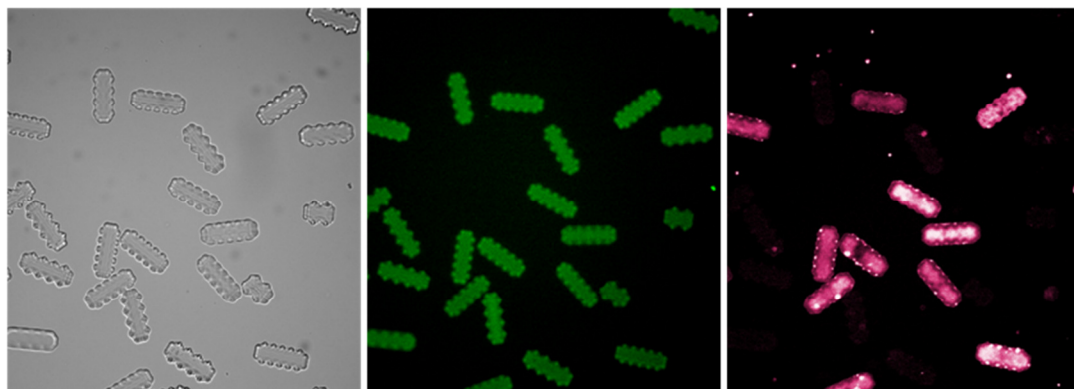
Figure 43. White light (left), SU-8 autofluorescence and Cy-5 fluorescence images of the multiplex analysis of a sample containing (TC) using immobilised probe DNA. The complementary probe (PC) was bound to type 3 particles (5 ridges visible) whilst the completely mismatching probe (PE) was bound to type 2 particles (4 ridges visible). Note only type 3 particles (complementary) exhibit Cy-5 fluorescence
