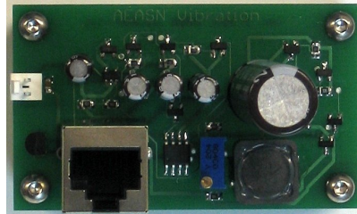
FIGURE 4.15: Circuit board for the vibration module.
