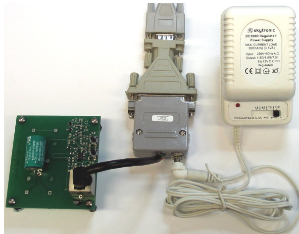
FIGURE 5.3: Set-up for EEDS on an energy module to be programmed over a 1-Wire interface, via a DS9097E COM port adapter connected to a PC serial port.
