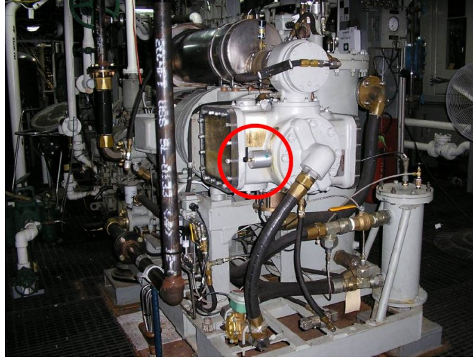
FIGURE 1.4: A S 5 NAP vibration powered sensor node mounted on an air compressor during a trial (reproduced from [6]).
