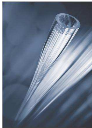
FIGURE 2.2: The capillaries stacked around a rod
