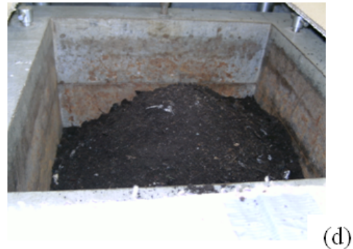
Figure 3. 30 - Sample preparation in 300 mm x 300 mm shear box (a) covered shear box to collect any MBT spilled during sample preparation (b) one of the levelled containers (c) Levelling of the MBT surface (d) after pouring the sample in to the shear box
