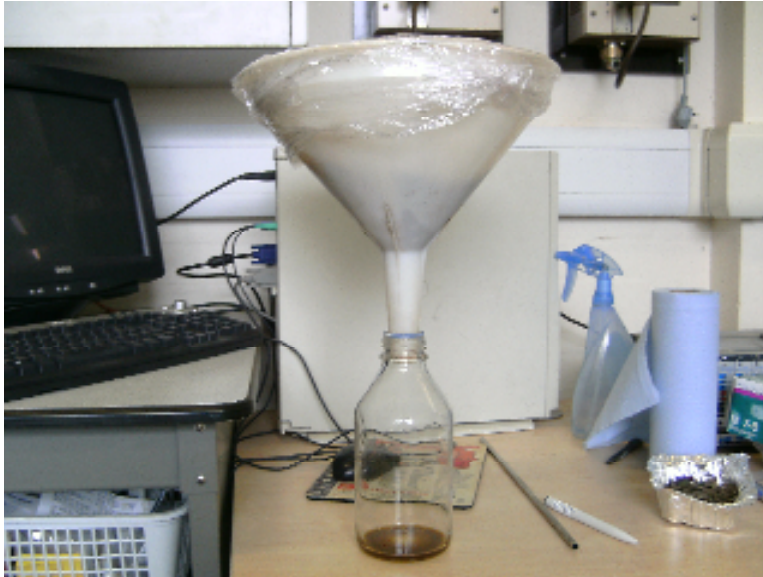
Figure 4. 9 - Apparatus used to obtain a field capacity sample
